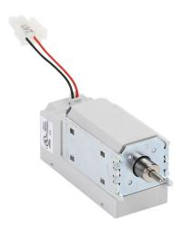
Gladiator field installable undervoltage trip, right side mount, 24 VAC/VDC sensing range, screw terminals. For use with Gladiator 800A and 1200A frame MCCBs.
