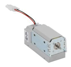
Gladiator field installable shunt trip, right side mount, 24 VAC/VDC coil voltage, screw terminals. For use with Gladiator 800A and 1200A frame MCCBs.
