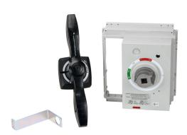
Gladiator rotary handle, tee, black, external front mount, 2-position, lockable in ON-OFF, defeatable, NEMA 3/3R/4. For use with Gladiator 800A and 1200A frame MCCBs. Operating mechanism included.
