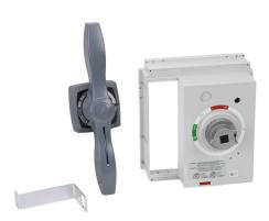
Gladiator rotary handle, tee, gray, external front mount, 2-position, lockable in ON-OFF, defeatable, NEMA 1/12. For use with Gladiator 800A and 1200A frame MCCBs. Operating mechanism included.
