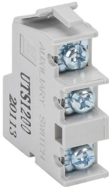
Gladiator field installable auxiliary contact, right side mount, (1) SPDT contact(s), 3A @ 250VAC/0.2A @ 250VDC, screw terminals, Auxiliary contact indicates if the MCCB is closed or open/tripped. For use with Gladiator 800A and 1200A frame MCCBs.
