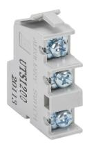
Gladiator field installable auxiliary contact, right side mount, (1) SPDT contact(s), 3A @ 250VAC/0.2A @ 250VDC, screw terminals, Auxiliary contact indicates if the MCCB is closed or open/tripped. For use with Gladiator 800A and 1200A frame MCCBs.
