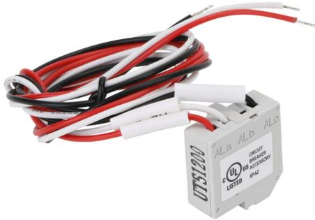
Gladiator field installable alarm contact, right side mount, (1) SPDT contact(s), 3A @ 250VAC/0.2A @ 250VDC, 20in 26AWG lead wires, Alarm contacts indicate when the MCCB is tripped. For use with Gladiator 800A and 1200A frame MCCBs.
