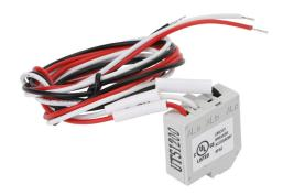
Gladiator field installable alarm contact, right side mount, (1) SPDT contact(s), 3A @ 250VAC/0.2A @ 250VDC, 20in 26AWG lead wires, Alarm contacts indicate when the MCCB is tripped. For use with Gladiator 800A and 1200A frame MCCBs.
