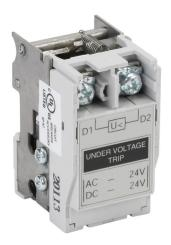
Gladiator field installable undervoltage trip, left side mount, 24 VAC/VDC sensing range, screw terminals. For use with Gladiator 150A to 600A frame MCCBs.
