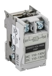
Gladiator field installable undervoltage trip, left side mount, 110-130 VAC/VDC sensing range, screw terminals. For use with Gladiator 150A to 600A frame MCCBs.
