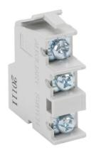
Gladiator field installable auxiliary contact, left or right side mount, (1) SPDT contact(s), 3A @ 250VAC/0.2A @ 250VDC, screw terminals, Auxiliary contact indicates if the MCCB is closed or open/tripped. For use with Gladiator 150A to 600A frame MCCBs.
