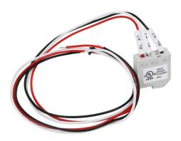
Gladiator field installable alarm contact, left or right side mount, (1) SPDT contact(s), 3A @ 250VAC/0.2A @ 250VDC, 20in 26AWG lead wires, Alarm contacts indicate when the MCCB is tripped. For use with Gladiator 150A to 600A frame MCCBs.
