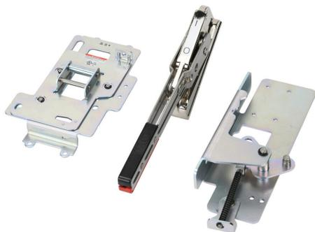
Gladiator flange handle, lever, chrome, external front mount, 2-position, lockable in OFF only, defeatable, NEMA 3/4/4X. For use with Gladiator 400A and 600A frame MCCBs. Operating mechanism included.
