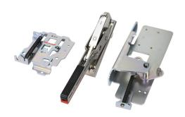
Gladiator flange handle, lever, chrome, external front mount, 2-position, lockable in OFF only, defeatable, NEMA 3/4/4X. For use with Gladiator 150A and 250A frame MCCBs. Operating mechanism included.
