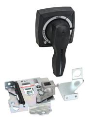
Gladiator rotary handle, pistol, black, external front mount, 2-position, lockable in ON-OFF, defeatable, NEMA 3/4/4X. For use with Gladiator 150A and 250A frame MCCBs. Operating mechanism included.
