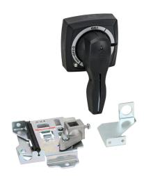
Gladiator rotary handle, pistol, black, external front mount, 2-position, lockable in ON-OFF, defeatable, NEMA 3/3R/4. For use with Gladiator 150A and 250A frame MCCBs. Operating mechanism included.
