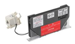
Gladiator field installable undervoltage trip, right side mount, 110-130 VAC/VDC sensing range, screw terminals. For use with Gladiator 100A frame MCCBs.
