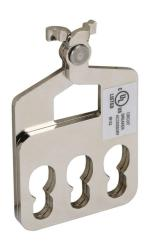
Gladiator lockout attachment, 5-8mm (3/16-5/16in) diameter. For use with Gladiator 100A frame MCCBs. For locking in the OFF position only. Accepts up to 3 locks.
