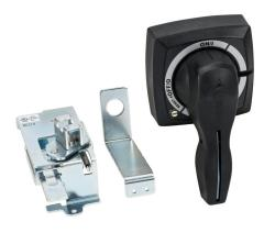
Gladiator rotary handle, pistol, black, external front mount, 2-position, lockable in ON-OFF, defeatable, NEMA 3/4/4X. For use with Gladiator 100A frame MCCBs. Operating mechanism included.
