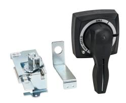
Gladiator rotary handle, pistol, black, external front mount, 2-position, lockable in ON-OFF, defeatable, NEMA 3/3R/4. For use with Gladiator 100A frame MCCBs. Operating mechanism included.
