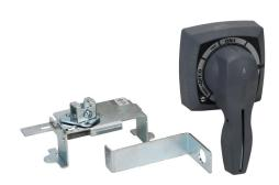
Gladiator rotary handle, pistol, gray, external front mount, 2-position, lockable in ON-OFF, defeatable, NEMA 1/12. For use with Gladiator 100A frame MCCBs. Operating mechanism included.
