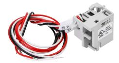
Gladiator field installable auxiliary contact, right side mount, (1) SPDT contact(s), 3A @ 250VAC/0.2A @ 250VDC, 20in 24AWG lead wires, Auxiliary contact indicates if the MCCB is closed or open/tripped. For use with Gladiator 100A frame MCCBs.
