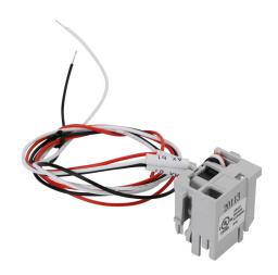
Gladiator field installable auxiliary contact, left side mount, (1) SPDT contact(s), 3A @ 250VAC/0.2A @ 250VDC, 20in 24AWG lead wires, Auxiliary contact indicates if the MCCB is closed or open/tripped. For use with Gladiator 100A frame MCCBs.
