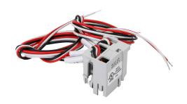
Gladiator field installable alarm/auxiliary contact, left side mount, (2) SPDT contact(s), 3A @ 250VAC/0.2A @ 250VDC, 20in 24AWG lead wires, Auxiliary contact indicates if the MCCB is closed or open/tripped. Alarm contact indicates if the MCCB is tripped.
