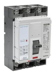
Gladiator molded case circuit breaker, 800A frame, 800A, 600 VAC, 3-pole, characteristics, adjustable electronic, 35kA @ 480 VAC interrupting rating, panel mount. Line and load lug terminals and terminal covers included.
