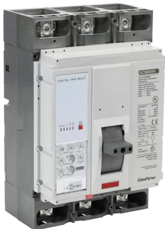
Gladiator molded case circuit breaker, 800A frame, 800A, 600 VAC, 3-pole, characteristics, adjustable electronic, 65kA @ 480 VAC interrupting rating, panel mount. Line and load lug terminals and terminal covers included.
