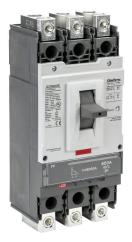
Gladiator molded case circuit breaker, 600A frame, 600A, 600 VAC / 600 VDC, 3-pole, characteristics, fixed thermal/fixed magnetic, 35kA @ 480 VAC interrupting rating, panel mount. Line and load lug terminals and terminal covers included.
