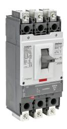
Gladiator molded case circuit breaker, 600A frame, 500A, 600 VAC / 600 VDC, 3-pole, characteristics, fixed thermal/fixed magnetic, 65kA @ 480 VAC interrupting rating, panel mount. Line and load lug terminals and terminal covers included.
