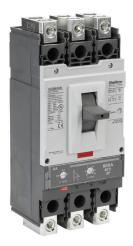
Gladiator molded case circuit breaker, 600A frame, 600A, 600 VAC / 600 VDC, 3-pole, characteristics, adjustable thermal/ adjustable magnetic, 65kA @ 480 VAC interrupting rating, panel mount. Line and load lug terminals and terminal covers included.
