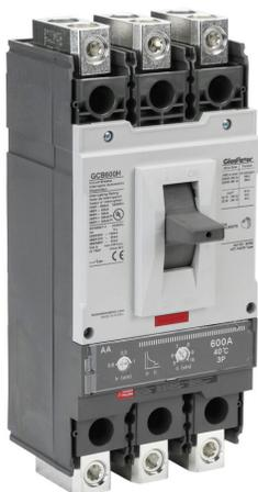
Gladiator molded case circuit breaker, 600A frame, 600A, 600 VAC / 600 VDC, 3-pole, characteristics, adjustable thermal/ adjustable magnetic, 65kA @ 480 VAC interrupting rating, panel mount. Line and load lug terminals and terminal covers included.
