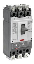
Gladiator molded case circuit breaker, 600A frame, 500A, 600 VAC / 600 VDC, 3-pole, characteristics, adjustable thermal/adjustable magnetic, 65kA @ 480 VAC interrupting rating, panel mount. Line and load lug terminals and terminal covers included.
