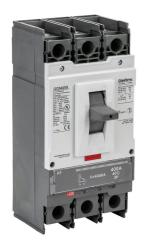
Gladiator molded case circuit breaker, 400A frame, 400A, 600 VAC / 600 VDC, 3-pole, characteristics, fixed thermal/fixed magnetic, 35kA @ 480 VAC interrupting rating, panel mount. Line and load lug terminals and terminal covers included.
