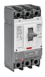
Gladiator molded case circuit breaker, 400A frame, 350A, 600 VAC / 600 VDC, 3-pole, characteristics, fixed thermal/fixed magnetic, 35kA @ 480 VAC interrupting rating, panel mount. Line and load lug terminals and terminal covers included.
