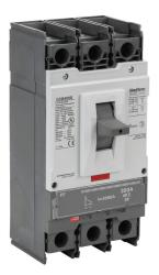
Gladiator molded case circuit breaker, 400A frame, 300A, 600 VAC / 600 VDC, 3-pole, characteristics, fixed thermal/fixed magnetic, 35kA @ 480 VAC interrupting rating, panel mount. Line and load lug terminals and terminal covers included.
