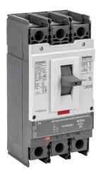
Gladiator molded case circuit breaker, 400A frame, 400A, 600 VAC / 600 VDC, 3-pole, characteristics, fixed thermal/fixed magnetic, 65kA @ 480 VAC interrupting rating, panel mount. Line and load lug terminals and terminal covers included.
