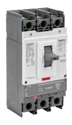
Gladiator molded case circuit breaker, 400A frame, 350A, 600 VAC / 600 VDC, 3-pole, characteristics, fixed thermal/fixed magnetic, 65kA @ 480 VAC interrupting rating, panel mount. Line and load lug terminals and terminal covers included.
