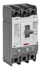
Gladiator molded case circuit breaker, 400A frame, 400A, 600 VAC / 600 VDC, 3-pole, characteristics, adjustable thermal/ adjustable magnetic, 65kA @ 480 VAC interrupting rating, panel mount. Line and load lug terminals and terminal covers included.
