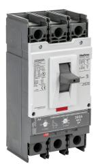
Gladiator molded case circuit breaker, 400A frame, 300A, 600 VAC / 600 VDC, 3-pole, characteristics, adjustable thermal/ adjustable magnetic, 65kA @ 480 VAC interrupting rating, panel mount. Line and load lug terminals and terminal covers included.
