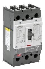
Gladiator molded case circuit breaker, 250A frame, 250A, 600 VAC / 600 VDC, 3-pole, characteristics, fixed thermal/fixed magnetic, 35kA @ 480 VAC interrupting rating, panel mount. Line and load lug terminals included.
