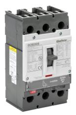
Gladiator molded case circuit breaker, 250A frame, 225A, 600 VAC / 600 VDC, 3-pole, characteristics, fixed thermal/fixed magnetic, 35kA @ 480 VAC interrupting rating, panel mount. Line and load lug terminals included.
