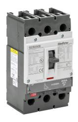
Gladiator molded case circuit breaker, 250A frame, 200A, 600 VAC / 600 VDC, 3-pole, characteristics, fixed thermal/fixed magnetic, 35kA @ 480 VAC interrupting rating, panel mount. Line and load lug terminals included.
