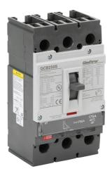
Gladiator molded case circuit breaker, 250A frame, 175A, 600 VAC / 600 VDC, 3-pole, characteristics, fixed thermal/fixed magnetic, 35kA @ 480 VAC interrupting rating, panel mount. Line and load lug terminals included.
