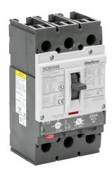
Gladiator molded case circuit breaker, 250A frame, 250A, 600 VAC / 600 VDC, 3-pole, characteristics, adjustable thermal/adjustable magnetic, 35kA @ 480 VAC interrupting rating, panel mount. Line and load lug terminals included.
