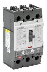
Gladiator molded case circuit breaker, 250A frame, 200A, 600 VAC / 600 VDC, 3-pole, characteristics, adjustable thermal/ adjustable magnetic, 35kA @ 480 VAC interrupting rating, panel mount. Line and load lug terminals included.
