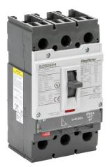
Gladiator molded case circuit breaker, 250A frame, 250A, 600 VAC / 600 VDC, 3-pole, characteristics, fixed thermal/fixed magnetic, 65kA @ 480 VAC interrupting rating, panel mount. Line and load lug terminals included.
