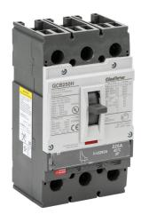
Gladiator molded case circuit breaker, 250A frame, 225A, 600 VAC / 600 VDC, 3-pole, characteristics, fixed thermal/fixed magnetic, 65kA @ 480 VAC interrupting rating, panel mount. Line and load lug terminals included.
