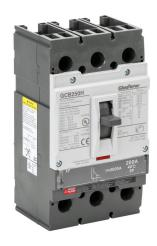
Gladiator molded case circuit breaker, 250A frame, 200A, 600 VAC / 600 VDC, 3-pole, characteristics, fixed thermal/fixed magnetic, 65kA @ 480 VAC interrupting rating, panel mount. Line and load lug terminals included.
