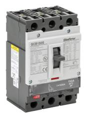
Gladiator molded case circuit breaker, 150A frame, 150A, 600 VAC / 600 VDC, 3-pole, characteristics, fixed thermal/fixed magnetic, 35kA @ 480 VAC interrupting rating, panel mount. Line and load lug terminals included.
