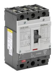
Gladiator molded case circuit breaker, 150A frame, 125A, 600 VAC / 600 VDC, 3-pole, characteristics, fixed thermal/fixed magnetic, 35kA @ 480 VAC interrupting rating, panel mount. Line and load lug terminals included.
