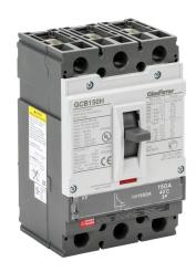
Gladiator molded case circuit breaker, 150A frame, 150A, 600 VAC / 600 VDC, 3-pole, characteristics, fixed thermal/fixed magnetic, 65kA @ 480 VAC interrupting rating, panel mount. Line and load lug terminals included.
