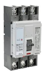
Gladiator molded case circuit breaker, 1200A frame, 1200A, 600 VAC, 3-pole, characteristics, adjustable electronic, 35kA @ 480 VAC interrupting rating, panel mount. Line and load lug terminals and terminal covers included.
