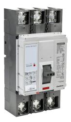
Gladiator molded case circuit breaker, 1200A frame, 1200A, 600 VAC, 3-pole, characteristics, adjustable electronic, 65kA @ 480 VAC interrupting rating, panel mount. Line and load lug terminals and terminal covers included.
