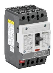
Gladiator molded case circuit breaker, 100A frame, 90A, 600Y / 480 VAC / 500 VDC, 3-pole, characteristics, fixed thermal/fixed magnetic, 35kA @ 480 VAC interrupting rating, panel mount. Line and load lug terminals included.
